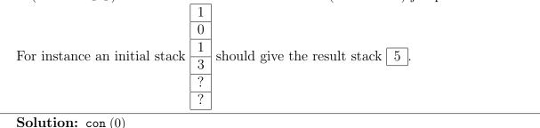
poke (0); init. result to 0  $\operatorname{con}(1)$ poke (1); init.  $2^i$  to 1 peek(1)mul; multiply with  $2^i$ peek(0)add ; add to result poke (0)peek(1); update multiplier  $\operatorname{con}(2)$ mul poke (1) con (1) 1; update digit counter peek(2)sub poke (2)peek(2); if counter = 0 go out cjp 4 jp - 26; else again poke(1) 1; clean stack and stop add halt
