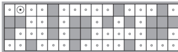
b) Possible robot locations after e_1 = \text{N S W} and e_2 = \text{N S}
