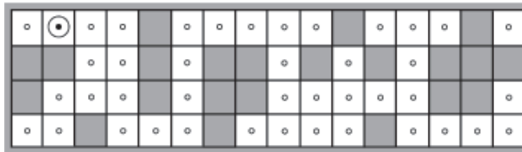
b) Possible robot locations after e_1 = N S W and e_2 = N S E
