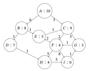
Every node is labeled with n : h(n) where n is the identifier of the node and h(n) is the heuristic for estimating the cost from n to a goal node. Every edge is labeled with its actual cost.
