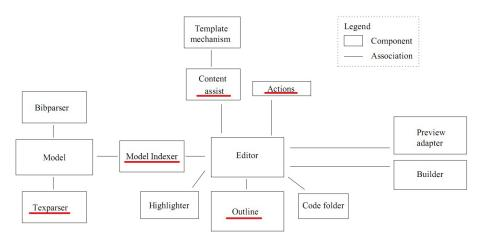
Fig. 3. Component architecture of TEXLIPSE (adapted from [?])
