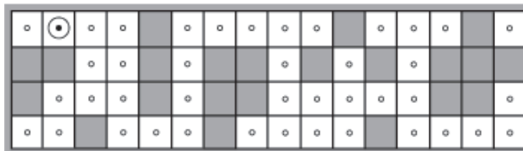
b) Possible robot locations after e_1 = N S W and e_2 = N S
